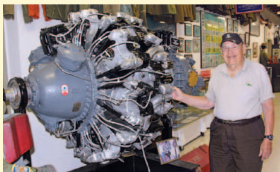
Ozzie with the museum's R-2800 Pratt and Whitney Double Wasp engine — the engine that powered the P-47 Thunderbolts
